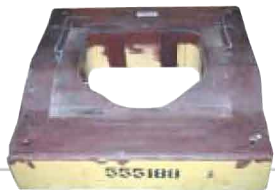
Part of car body, DCo5, s_0 = 1.75 mm; 300 parts
