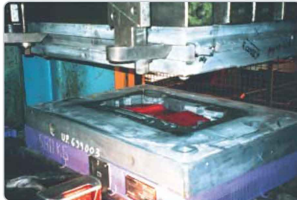
ebalta tooling resins for sheet metal forming give excellent gliding properties - ideal for saving lubricants and forming coated sheet metal
