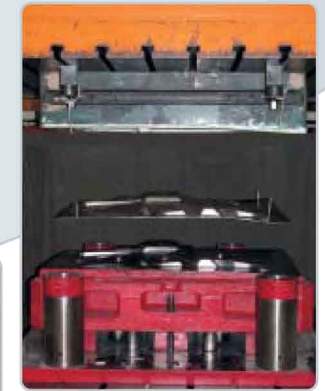
Door inner part, AA 6016, s_0 = 1.0 mm; 1,000 parts
