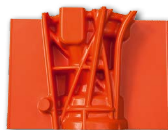
Foundry pattern made of ebaaboard 1220.
