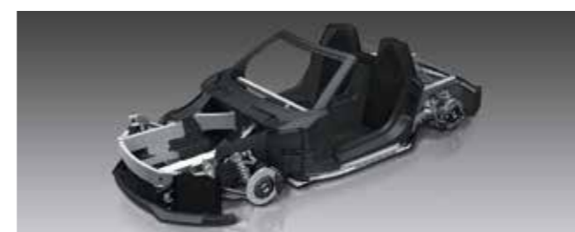
Roding CFK-chassis made of AH 140 from vacuum infusion
