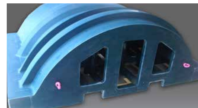
Master model for prepreg tool made of ebablock® P 185. Size: 3760 x 2990 x 1640 mm, volume: 3000 litres
